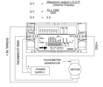
Since the division factor falls between 1.2 and 10.5, DIP switch position S2 is set to the "ON" position, according to the Division Factor Selection Chart.
